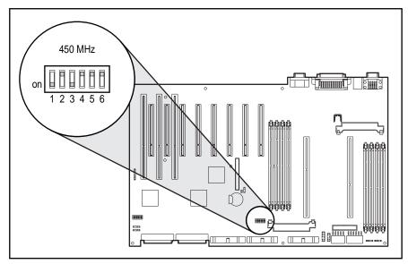
Figure 4-6. 450 MHz processor switch location and default settings
